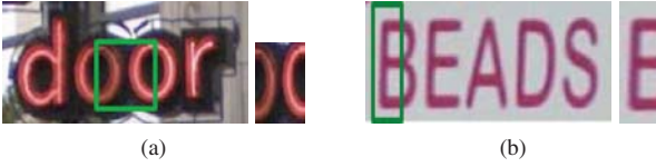
Figure 3: Typical challenges in multi-class character detection. (a) Inter-character confusion: A window containing parts of the two o’s is falsely detected as x. (b) Intra-character confusion: A window containing a part of the character B is recognized as E.
