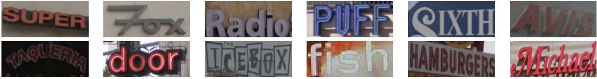
Figure 2: Scene text often contains examples that have a large variety of appearances. Here we show a few sample images from the SVT [30] and ICDAR [1] datasets, with issues such as, very different fonts, shadows, low resolution, occlusions. These images are much more complex than the ones seen in typical OCR datasets. Standard off-the-shelf OCRs perform very poorly on these datasets [23, 29].
